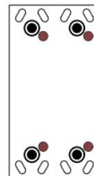
TFA L = 80 mm 2 × 4 bars with a diameter of 6 mm L = 400 mm
