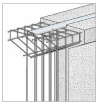
• HPTR channels are cast flush to the surface. The concrete surface should be trowelled smooth enabling the metal sheets to be positioned directly over the channels.
