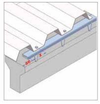
• The minimum edge spacing (ae) should be no less then 20 mm. The distance (x) between the channel end the screw position should be no less than 25 mm.
