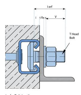
l erf = Bolt length i = channel lip thickness
