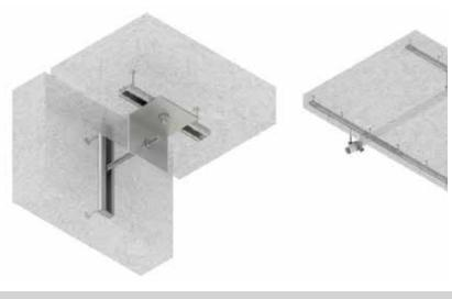
· Connection of concrete beams
