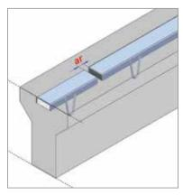
• The minimum spacing (ar) between channels should be 20 mm.
