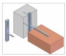
• Lugs are prepunched on the back of the channel at 250 mm centres. The lugs are easily bent out on site prior to the casting of concrete.
