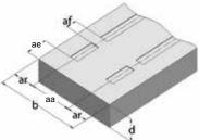
Execution 2 : Can be cut into two pieces at the centre. Edge spacing must be minimum 75 mm.
