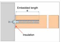
• Wall ties can be used for masonry wall connections fixed to load bearing walls. Embedding length (e) is achieved with the length of the wall tie.
