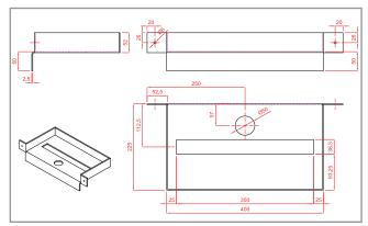
HAZ-RBX Recess Box Anchor channels can be custom made. The above dimensions (mm) are for HMPR -CE- 49/30-350 type channel
