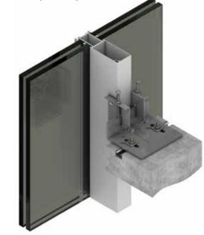
Curtain wall fixing at the edge of floor slab
