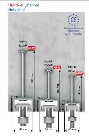
HMPR Hot rolled channels are suitable to with stand dynamic loads as well as static loads. These channels are available in hot dip galvanized and mild steel finish 1.0038 (S235JR)
