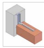
• HWT wall ties can be used with cast in channels type 28/15 and 38/17.
