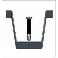
• Fixing is done with self drilling screws on to the HPTR cast in channels, without the need of pre-drilled holes. Power screw driver with 1500 rpm is required for fixing.
