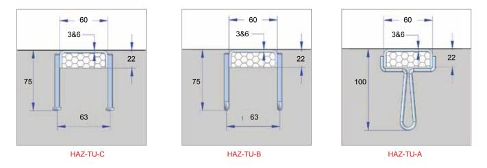
HAZ-TU Cast in channels for profiles metal sheet installations are supplied in either 3 or 6 mm thicknesses. A foam filler is inserted in the open slot of the channel for preventing inflow of wet concrete during casting. There are studs welded on to the channel for strong connections on to the concrete. There are three different stud versions which offer different results for loads and minimum edge spacings. Channels are supplied in Stainless steel and hot dip galvanized mild steel.
