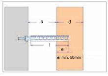
• Wall ties can be used on masonry facade cladding. A minimum embedded length of 50 mm should be applied. The embedded length (e) is determined by correctly setting the length of the wall tie (L) and the masonry block width (d).
