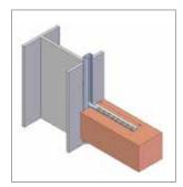
• HMP channels can be welded on to structural steel to allow wall tie connections.
