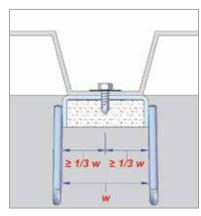
• Drilling positioning should be made in the middle of the channels, leaving a minimum distance 1/3 of the width from the side of the channel.
