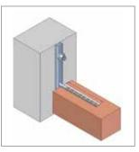
Connections on to surface fixed HMP channels type 28/15 and 38/17 can also be made.
