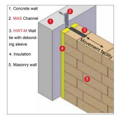
Wall ties are easily inserted into the debonding sleeves before installation is made.
