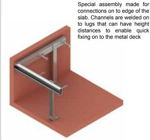
slab. Channels are welded on to lugs that can have height distances to enable quick
